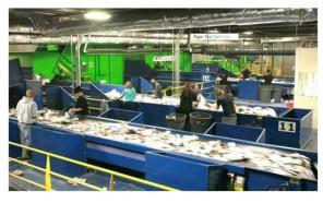
There, the materials are loaded onto conveyor belts where employees in pre-sort lines manually remove large metal, plastic or paper items as well as anything that might be harmful including plastic bags, sharps, rope and trash. Glass is removed early in the process to prevent damage to the conveyor belts and equipment.
